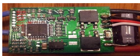
Fig 3: Internal Circuit of Electronic Speed Controller
